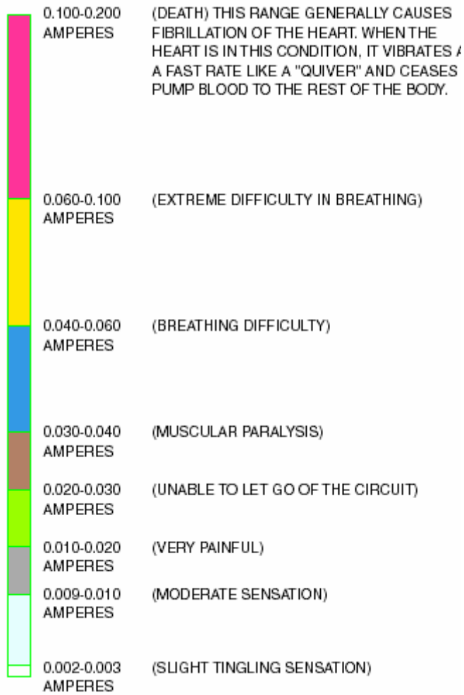
FIGURE S-1 The effects of electric current on the body
